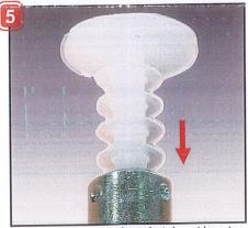
Put the cap into the piece, but do not insert it entirely (in order to protect the internal thread)
