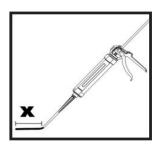
Remove the threaded cap from the cartridge. Tightly attach the mixing nozzle. Do not modify the mixer in any way. Made sure the mixing element is inside the mixer. Use only the supplied mixer. Insert the cartridge into the dispenser gun. Discard the initial trigger pulls of adhesive. Discard the first 10ml of resin.
